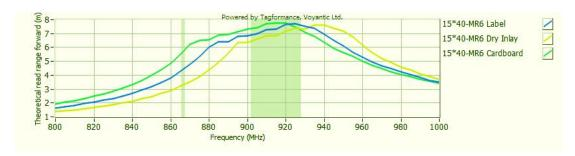
Sensitivity&Read Range Test power: 4W EIRP
